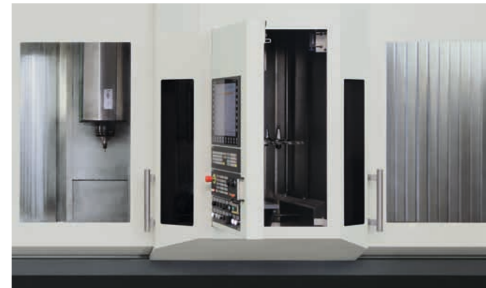
The tool changer is located behind the control panel
