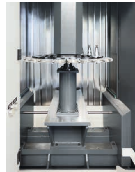
The plate changer is easily accessible from the front
