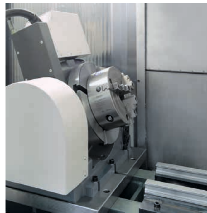
2 axes NC-tilting rotary table from AXA with continuous 360° round axis and tilting axis from 0° to 90°
