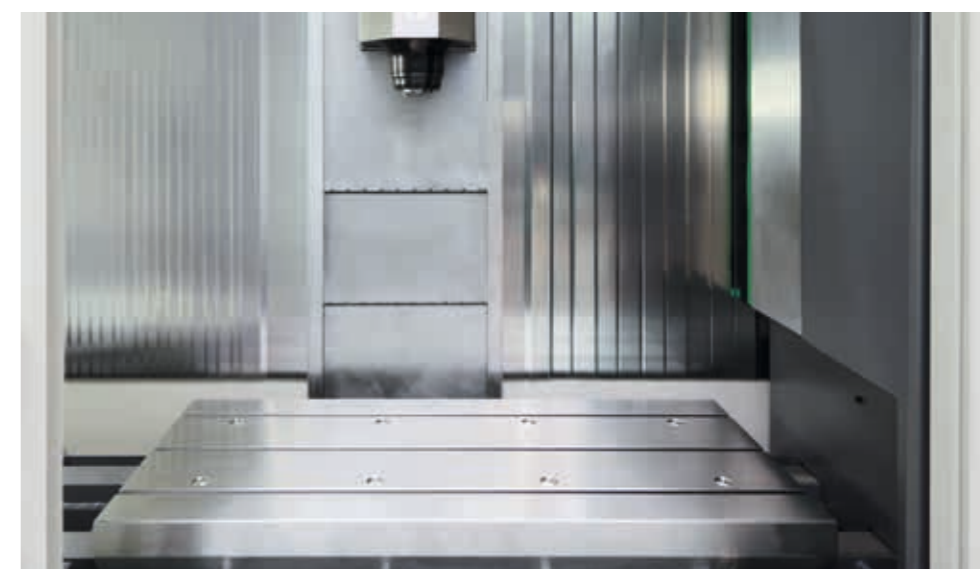
Custom working area for passing long work pieces beneath the tool changer
