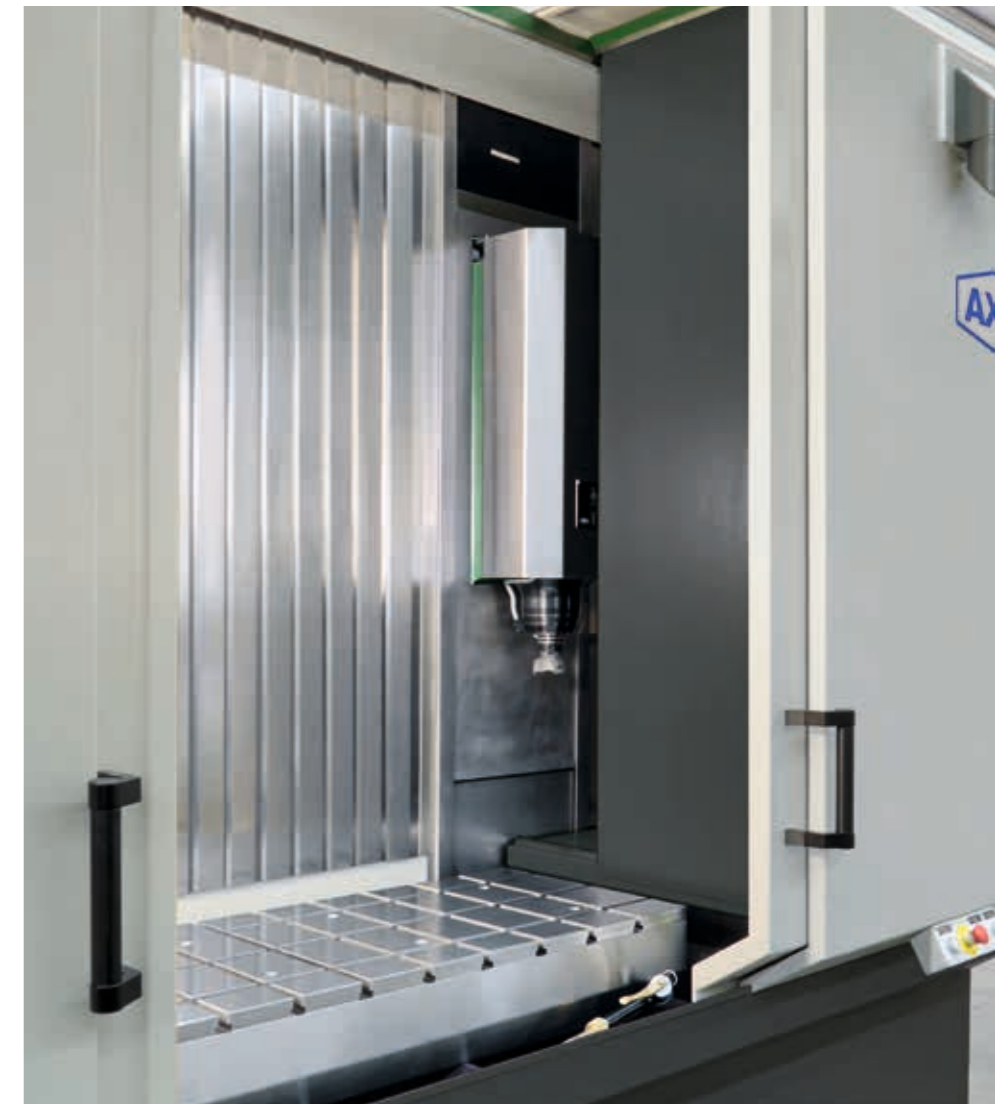
Compact and uncluttered workspace with direct spindle access to the tool magazine
