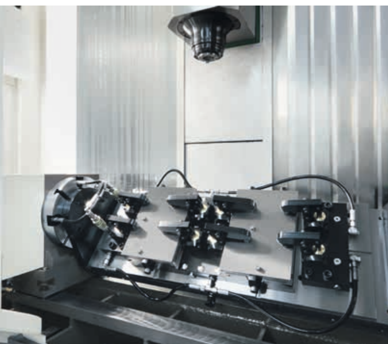
Rotary table with counter bearing and swivel bridge for mechanical multiple clamping system
