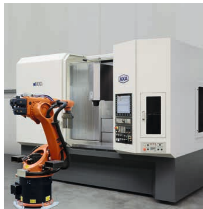
Installed industrial robot in front of the travelling column machine for direct machine loading and unloading with workpieces
