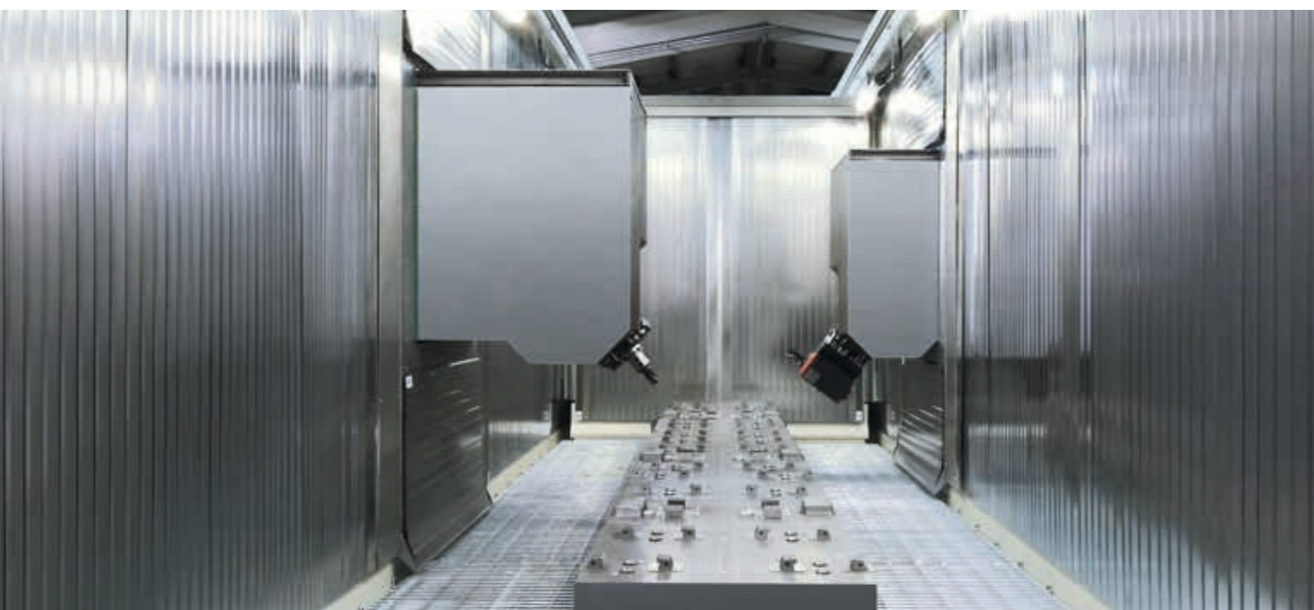
Main spindles that swivel around the X axis enable flexible manufacture of any contours, including with inclinations
