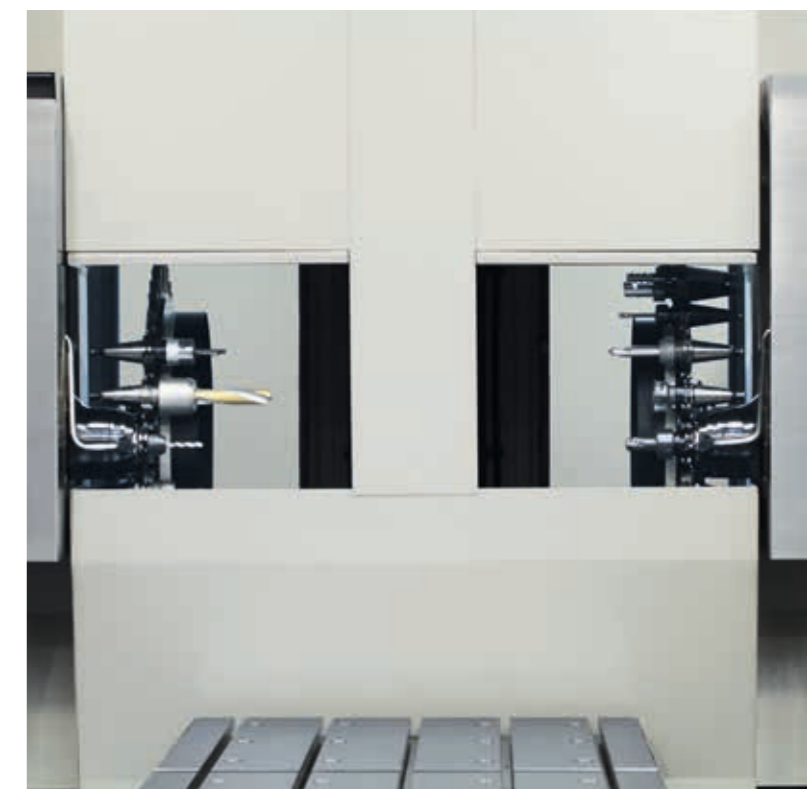
Two horizontal tool plate changers are in place at the face end
