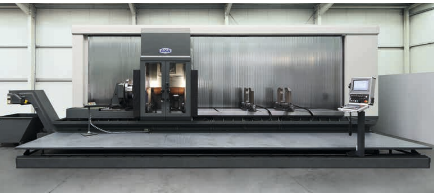
Instead of the fixed machine cladding of the heavy travelling column machining centre with tilting head, the working space around the spindle is encased in a hood that moves with the travelling column
