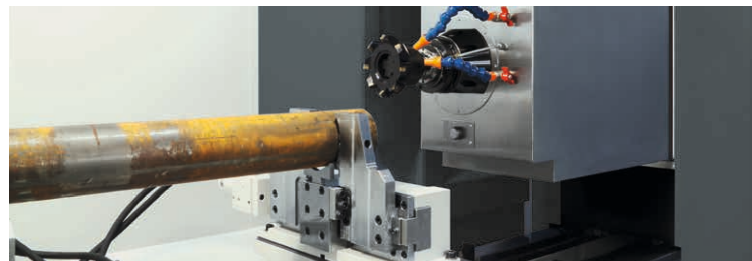
A universal spindle is used, which has been adapted to the machining task
