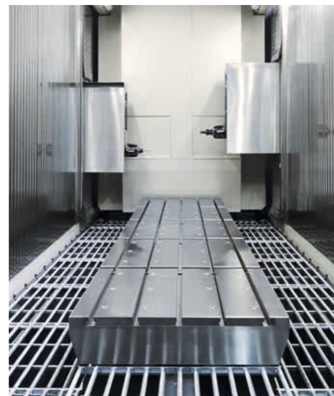
The clamping table is located centrally between the two travelling columns
