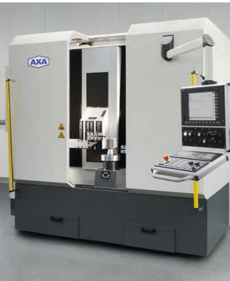
Vertical integration of the turning spindle for good chip flow and simple manual or automatic parts feed
