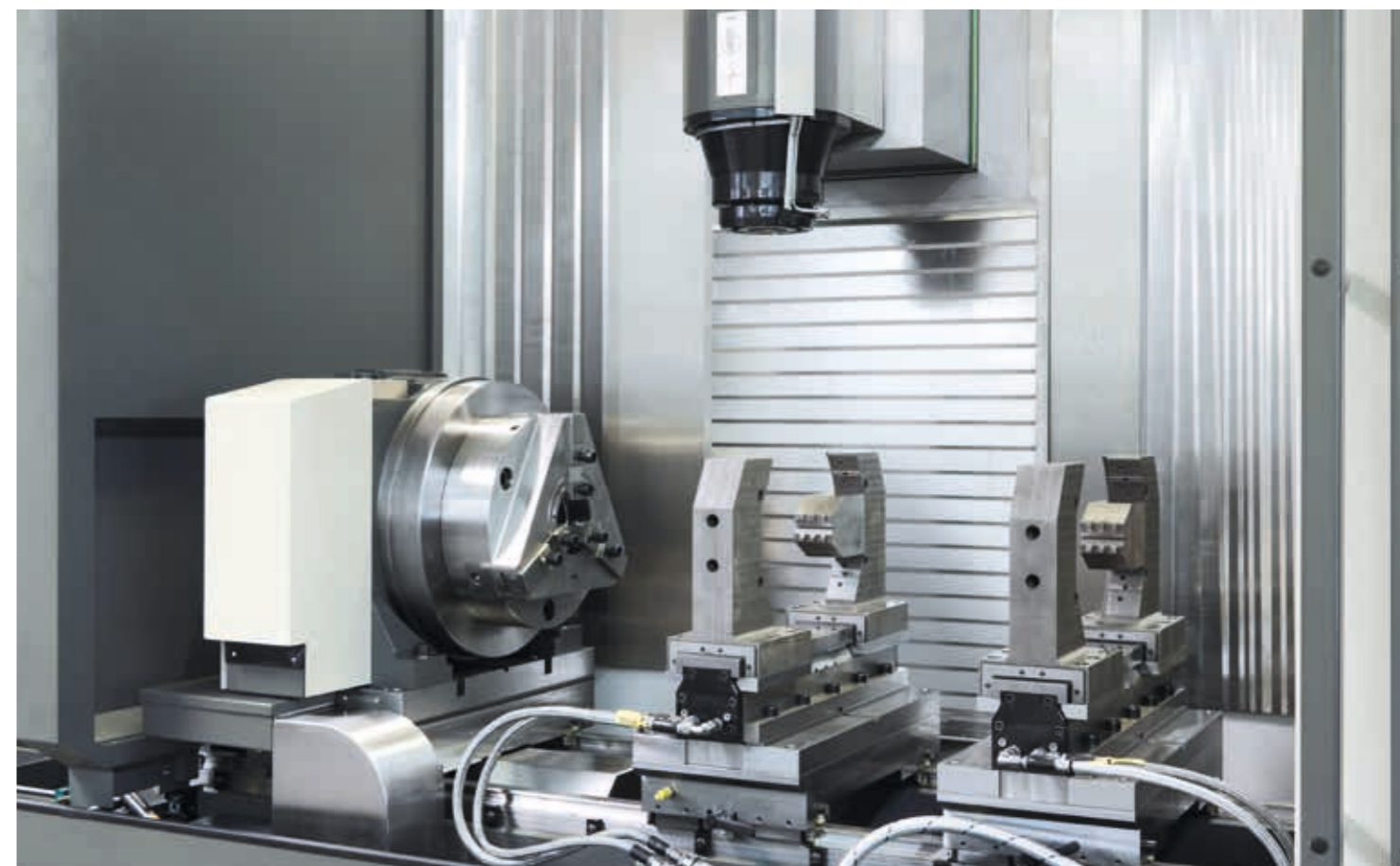
Shafts and pipes are held in centring clamps – The workpieces are automatically rotated by means of the rotary table housed on the left-hand side and the tailstock installed on the right-hand side
