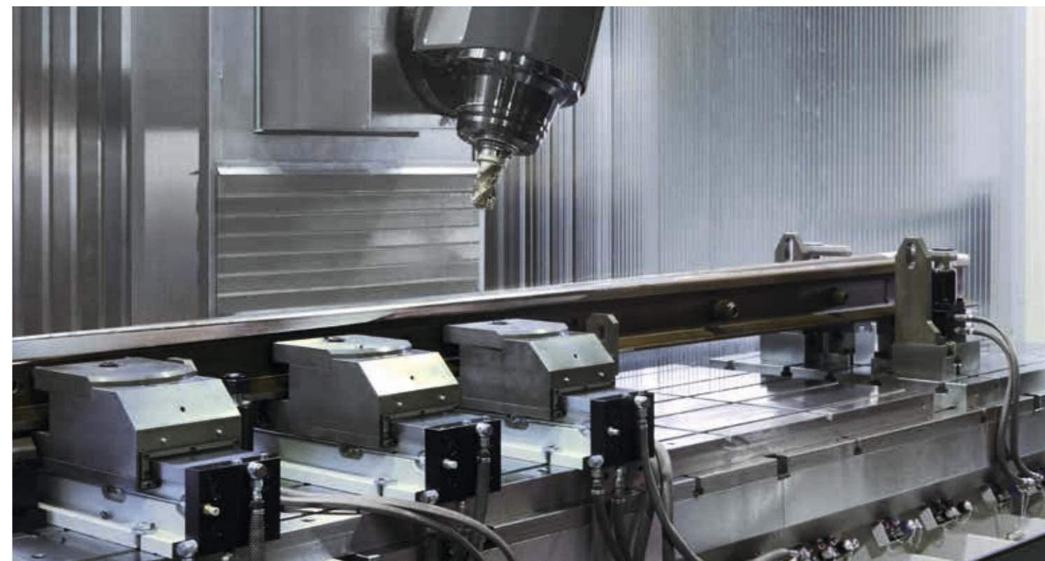
In the right hand working space long strips can be manufactured in clamps that can be positioned flexibly
