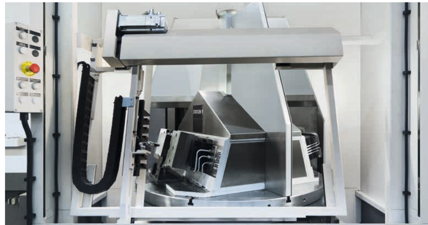
By pivoting the indexing table through 180° the ready-machined workpiece is rotated into the setup position while the next raw workpiece is simultaneously rotated into the machining position
