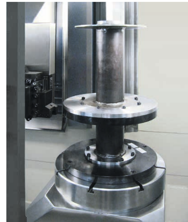
A rotary axis driven by a torque motor is used as a turning spindle
