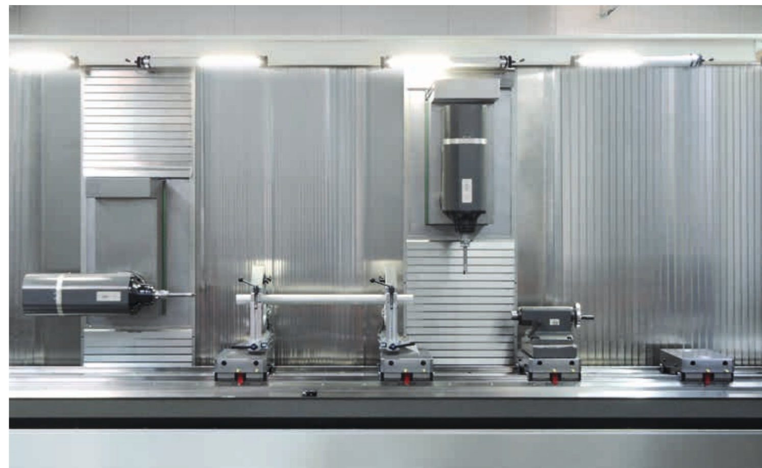
The table area is equipped with guide rails on which support units with rotary tables, clamping shells and tailstocks can be flexibly fitted and positioned
