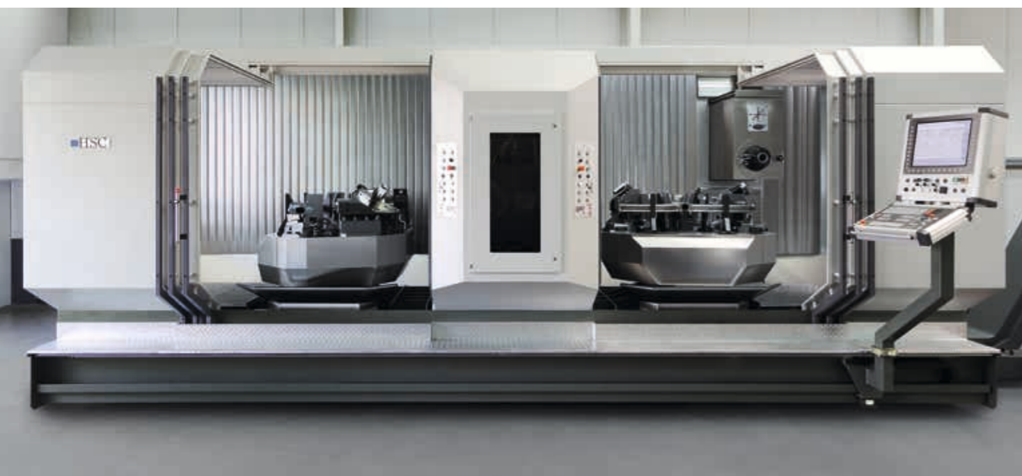
Two working spaces with one rotary table each, separated by a centrally assembled tool changer, enable clamping and cutting on one machine during machining
