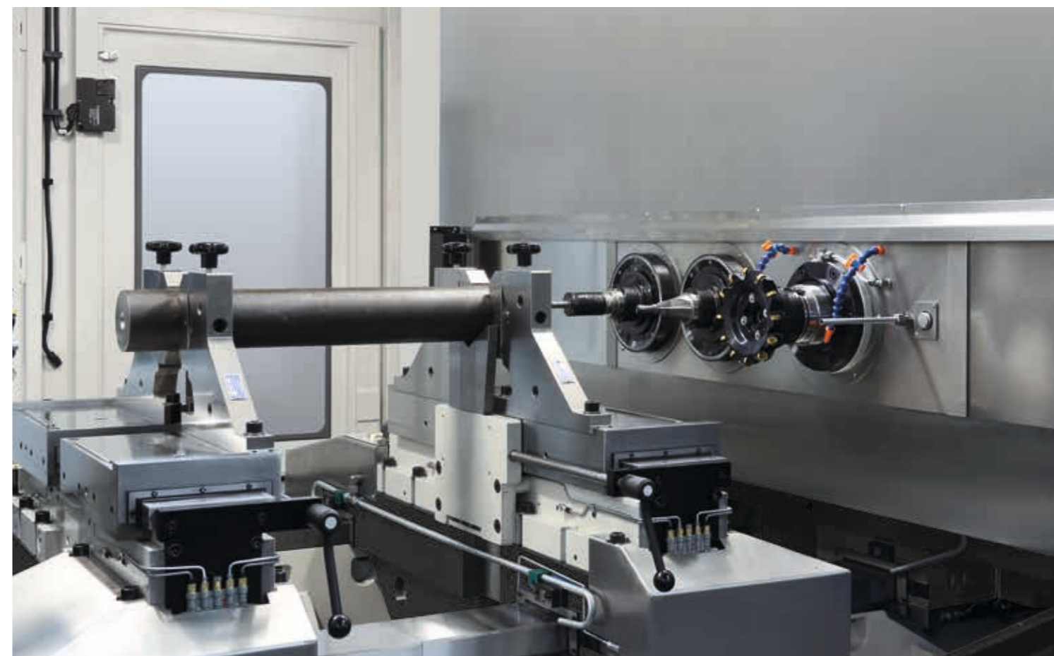
The machine is adjusted for different tool diameters by exchanging the clamp jaws and pre-centring on the centring vices
