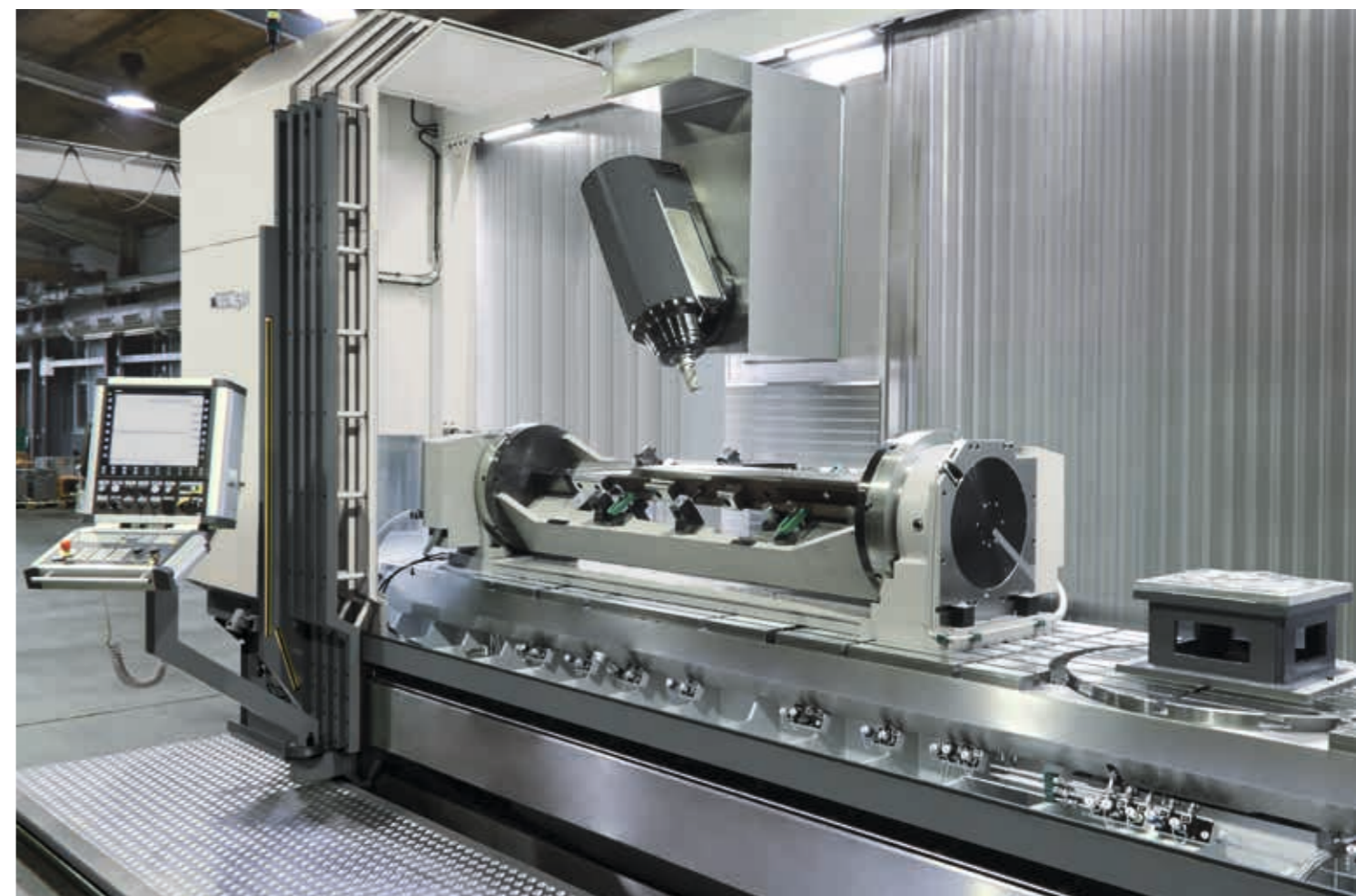
Two NC rotary tables working in gantry mode ensure torsionally stiff suspension of the long clamping bridge in the left-hand pendulum working space
