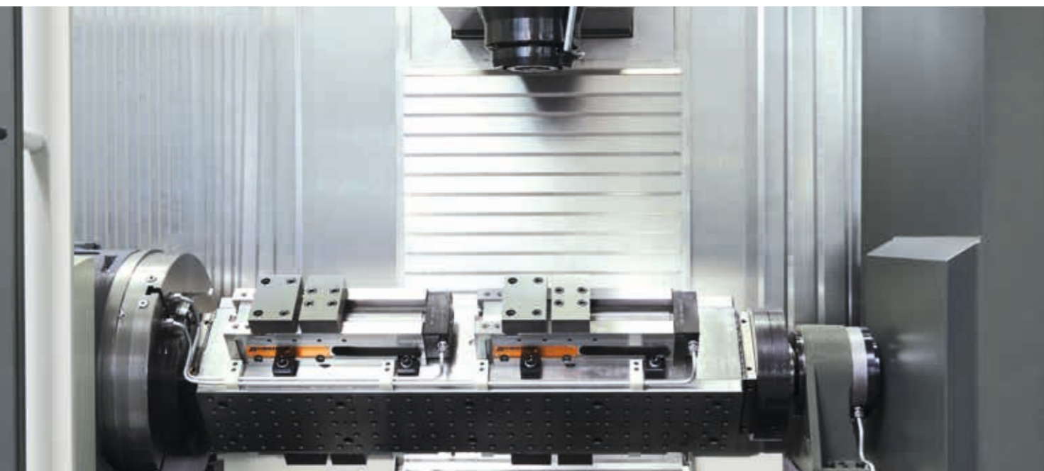
On the swivelling bridge installed in the left-hand pendulum working space, several workpieces can be clamped in parallel and each machined on three sides
