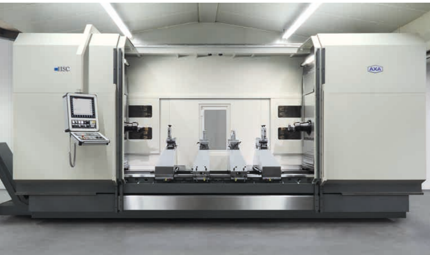
The ends of long workpieces are machined on a horizontal centre with two main spindles opposite one another which can be moved along the X-, Y-, or Z-axis
