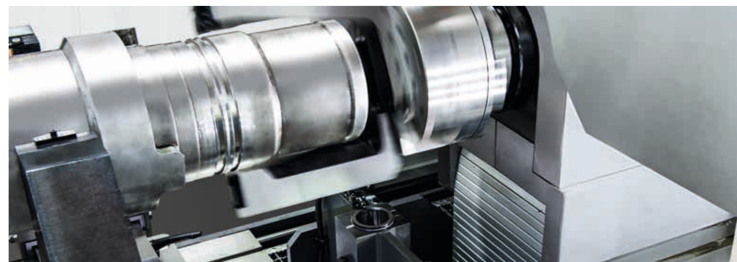
External machining of the sealing surfaces
