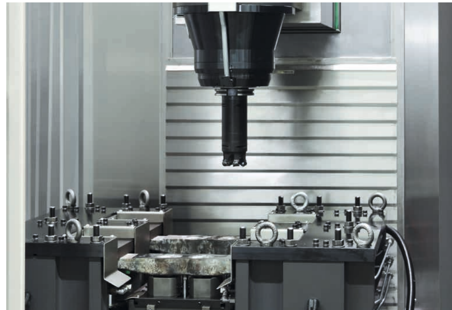
Parallel machining of two workpieces – These are aligned by means of centring bolts and clamped from beneath against a hydraulically movable surface
