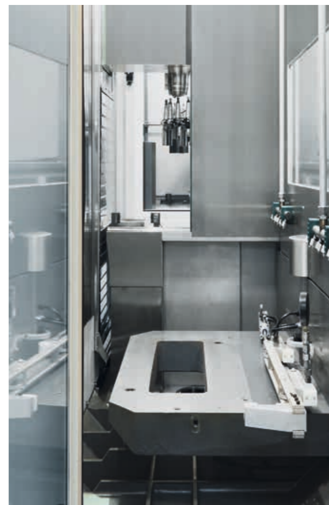
The rear working space has been optimised for machining abrasive materials, with mains water used as the coolant
