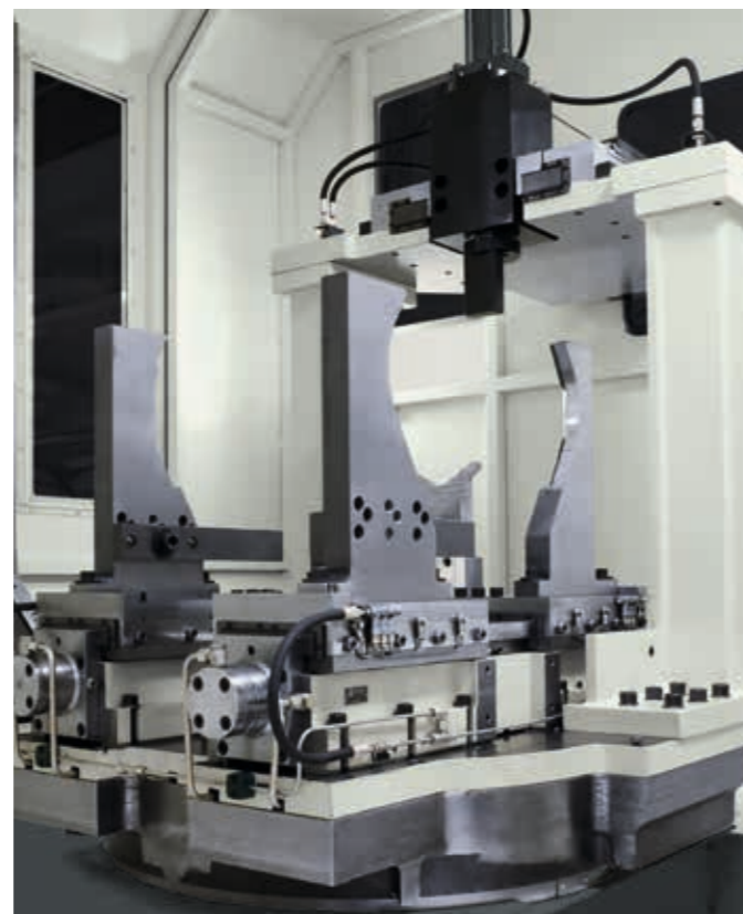
Centering clamps ensure that pipes are clamped centrally – Top jaws are swapped according to the different pipe diameters
