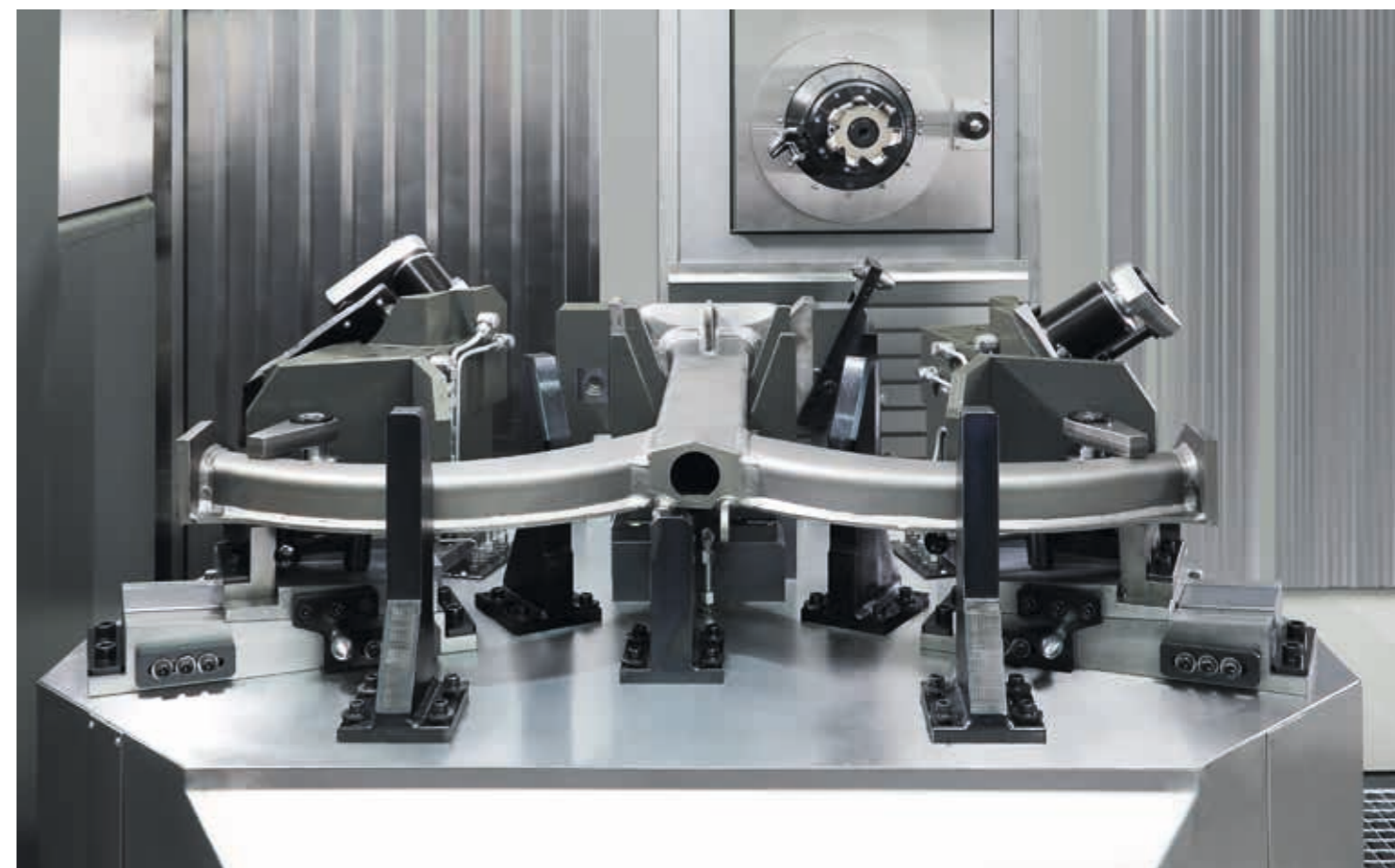
The assembly of the clamping device and workpiece on a rotary table allows several sides to be machined in one clamping operation
