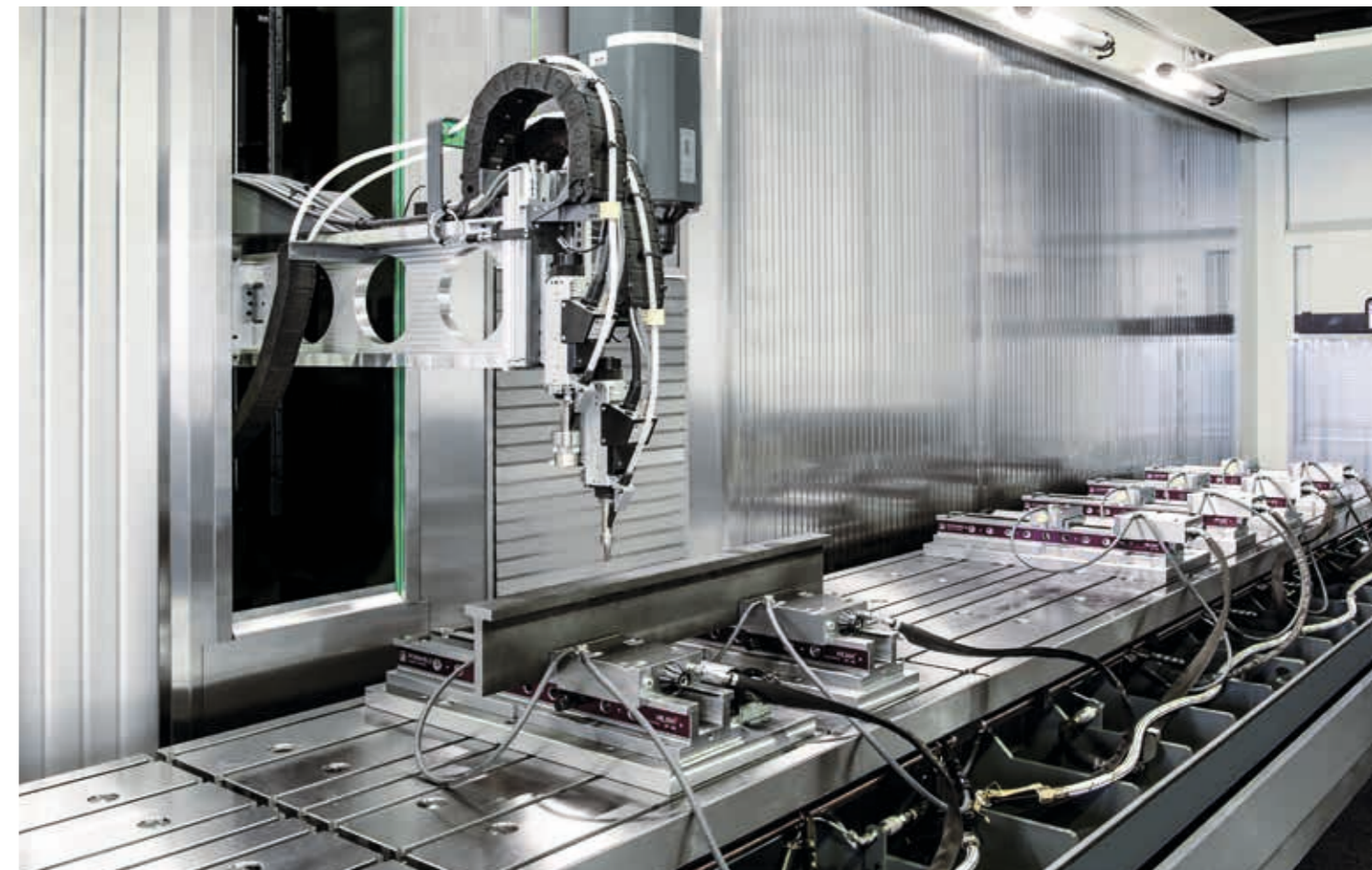
Two welding heads that are independently movable along the Y- and Z-axis move with the travelling column – These are used to weld threading bolts that are automatically supplied by a magazine moving with them
