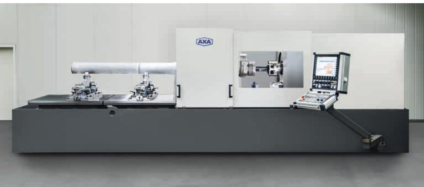
One-sided post-machining of sealing surfaces on long pipes
