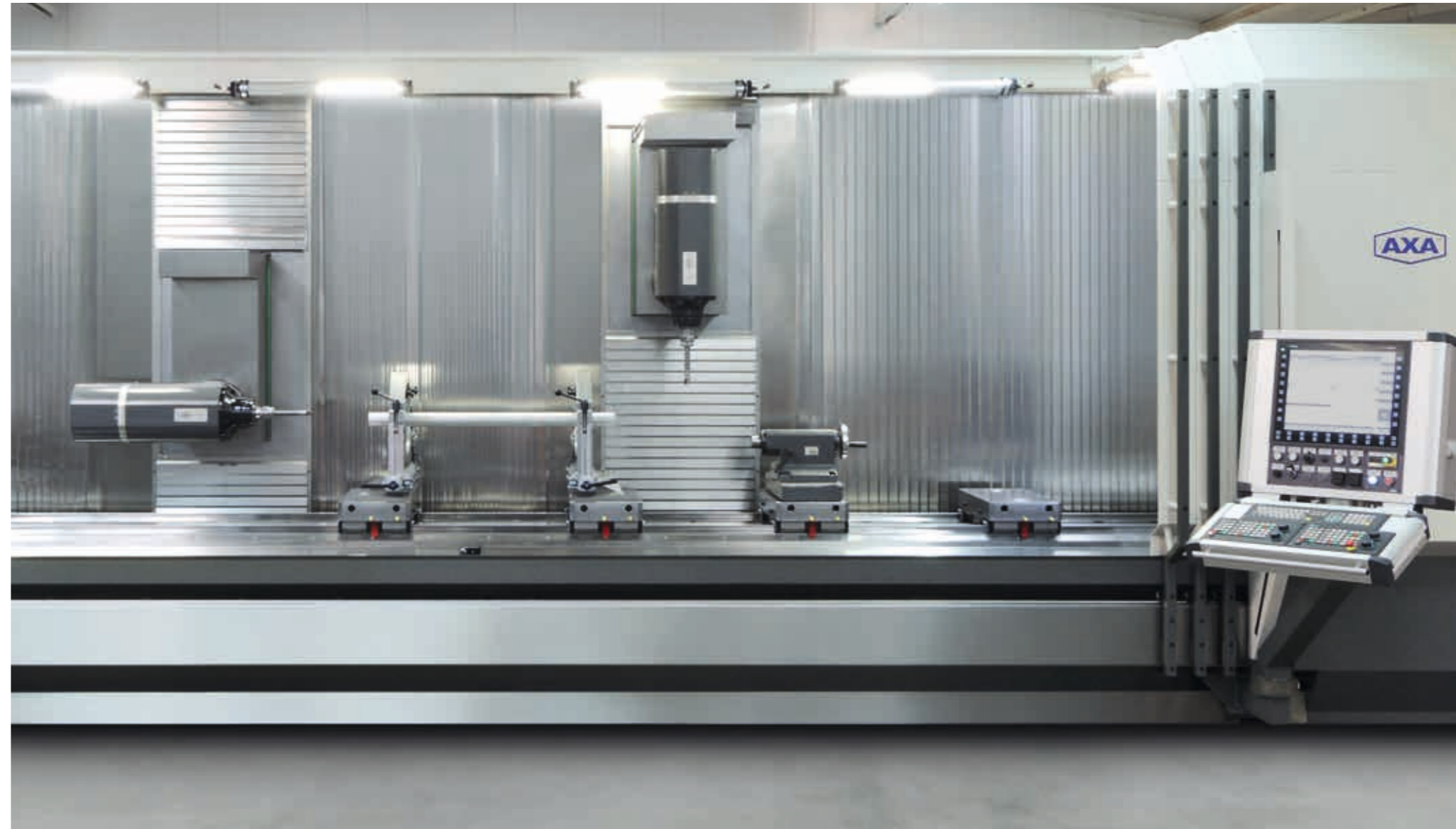
The parallel machining of a workpiece with double travelling column machining centre reduces the production time by up to 50% - the time-consuming long strokes are no longer required during face-side machining
