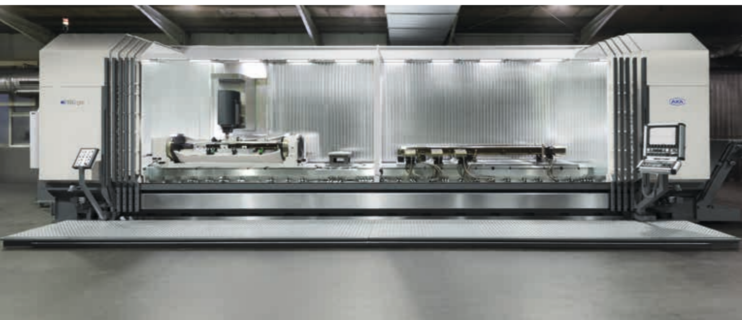
The heavy SK 50 pendulum machining centre is fitted with a high-performance tilting spindle head – Different clamping devices allow different workpieces to be machined in parallel
