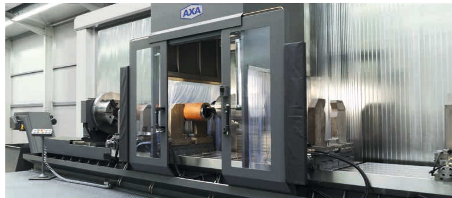
During the setup, the spindle is accessible through the opened doors of the hood that moves with the travelling column – Safety buffers attached to the side of the hood serve as protection against impact
