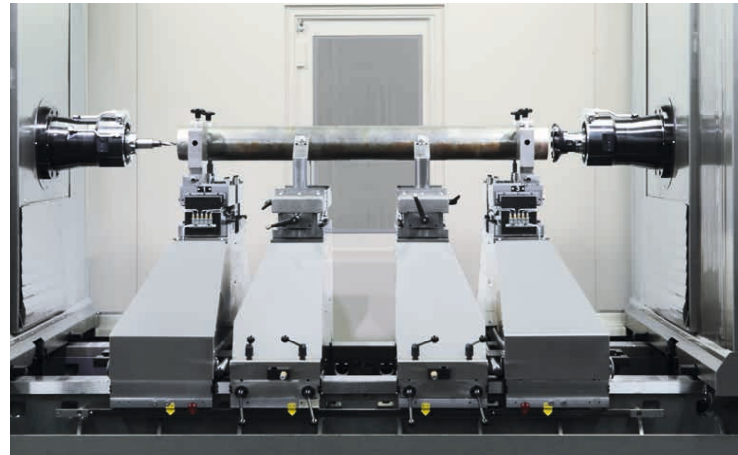
As well as the centring clamps on the ends of the shafts, intermediate supports are used to improve the stability
