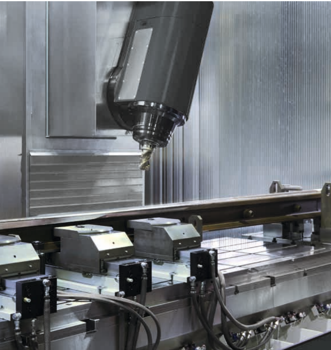
Adjustably placed hydraulic vice enable the secure and variable tension of long rails
