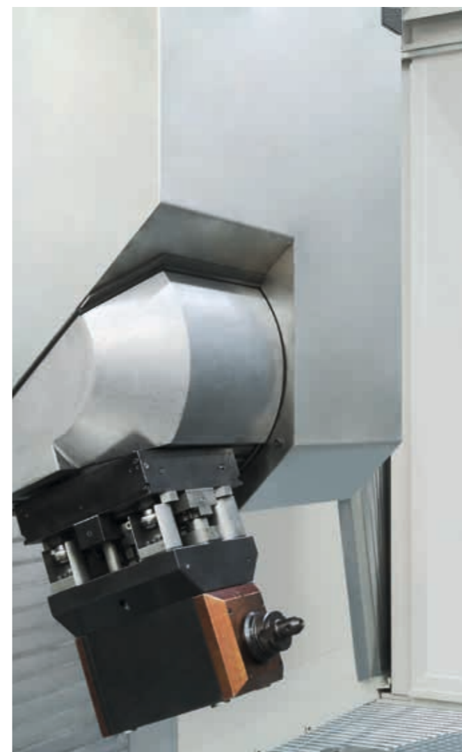
Partial machining from beneath by bolting heavy angular milling heads above a four-point support
