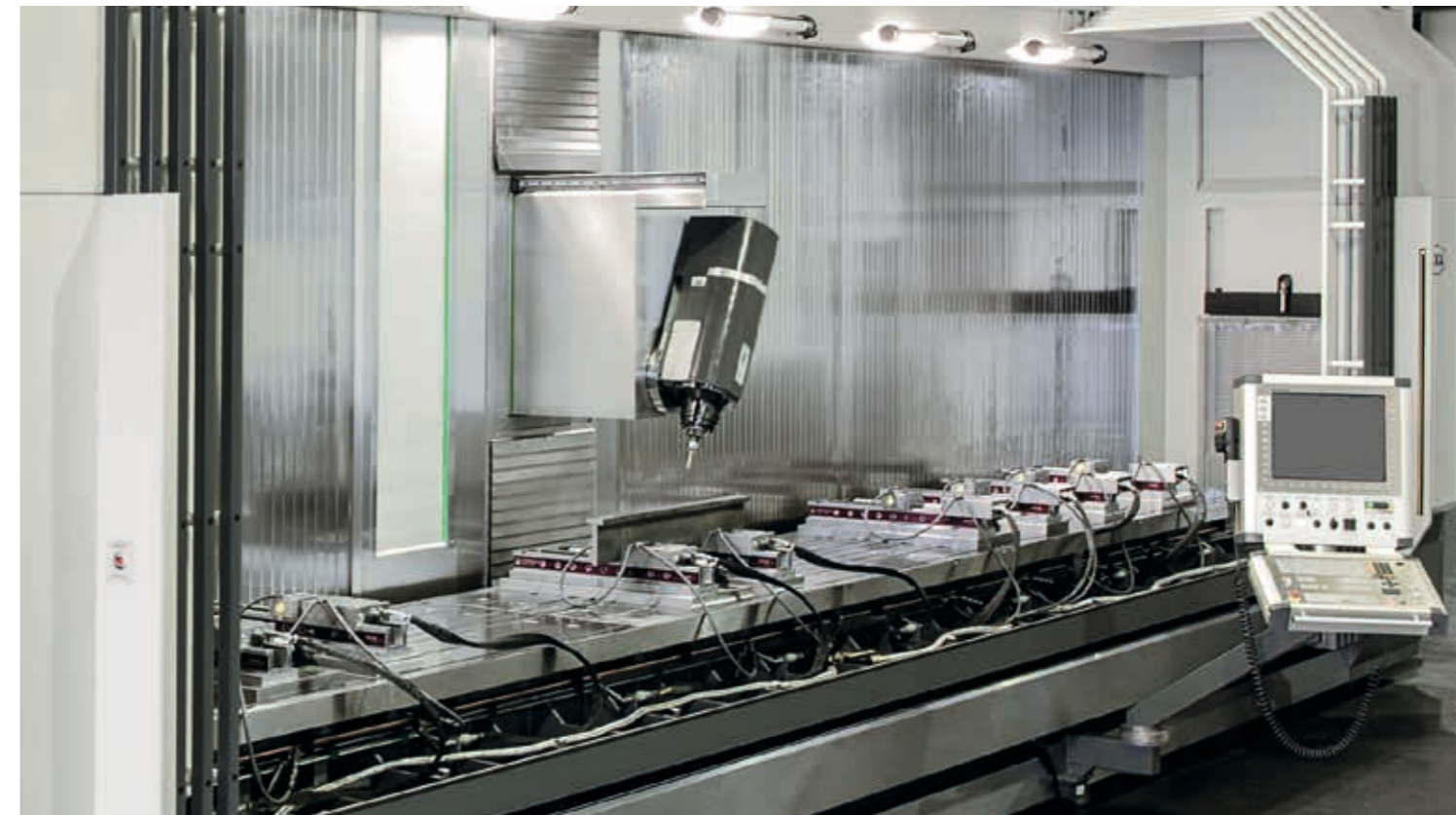
The girders are held in movable hydraulic clamps aligned with the machine table
