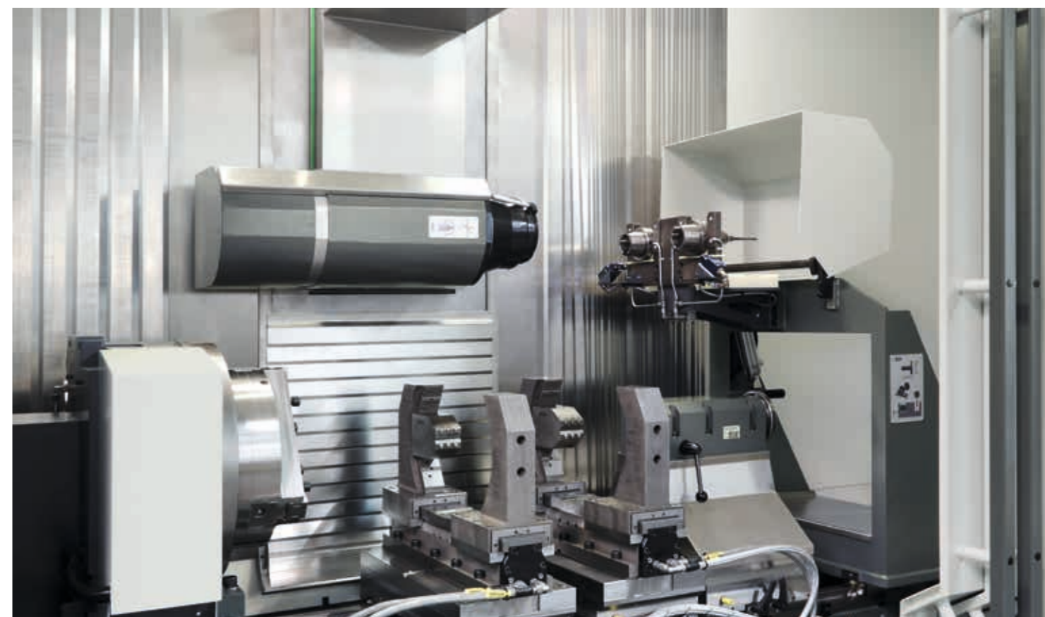
Use of special tools on a horizontally aligned pick-up magazine
