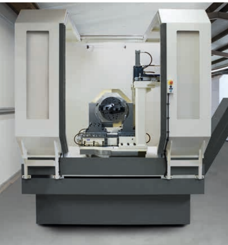
Centering clamps ensure that pipes are clamped centrally – Top jaws are swapped according to the different pipe diameters
