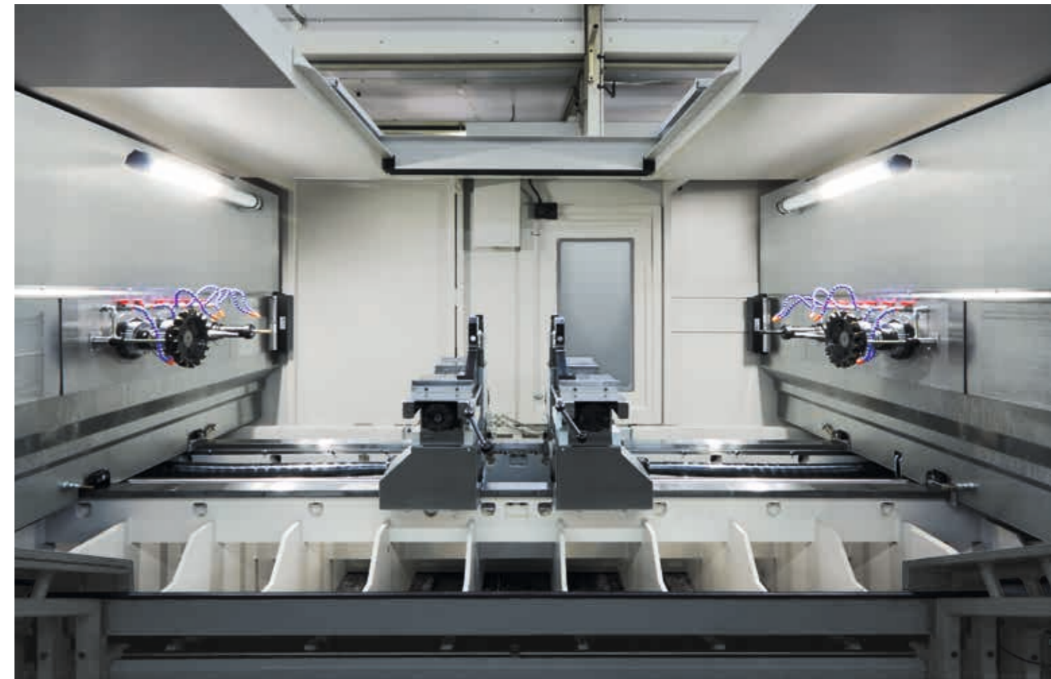
The double end machining centre consists of two Z-slides positioned opposite one another with tool supports both movable on the X-axis
