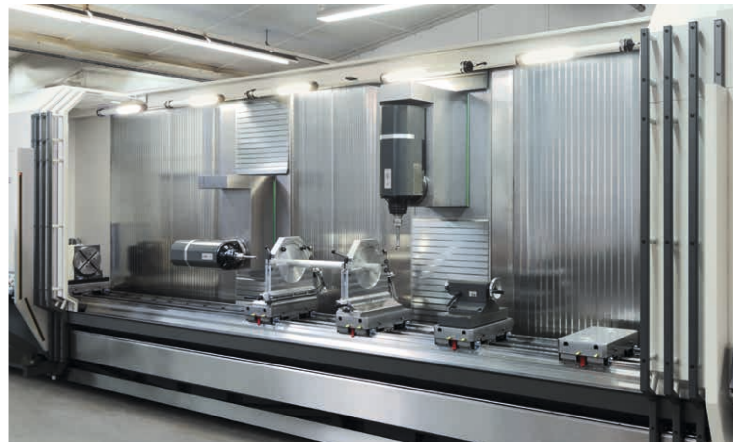
Using the rotary table and tailstock, the workpieces can be rotated in position in addition to the tilting spindle heads
