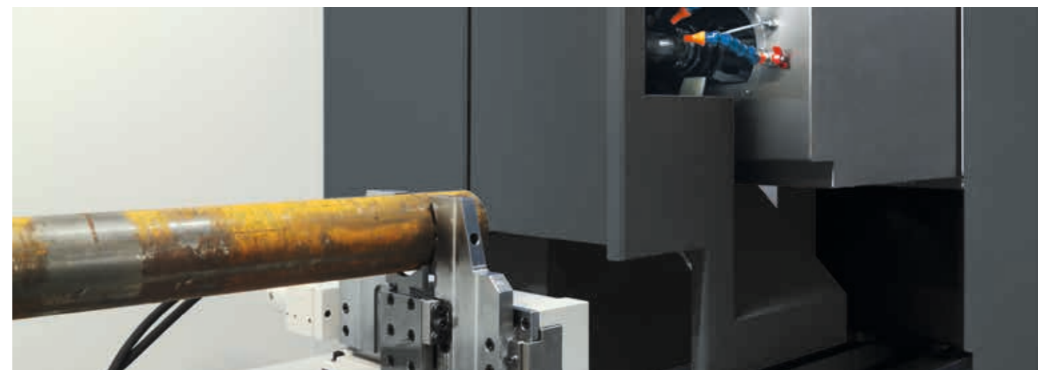
A tool plate changer set up alongside the spindle makes a wide variety of tools available for the flexible machining of shafts
