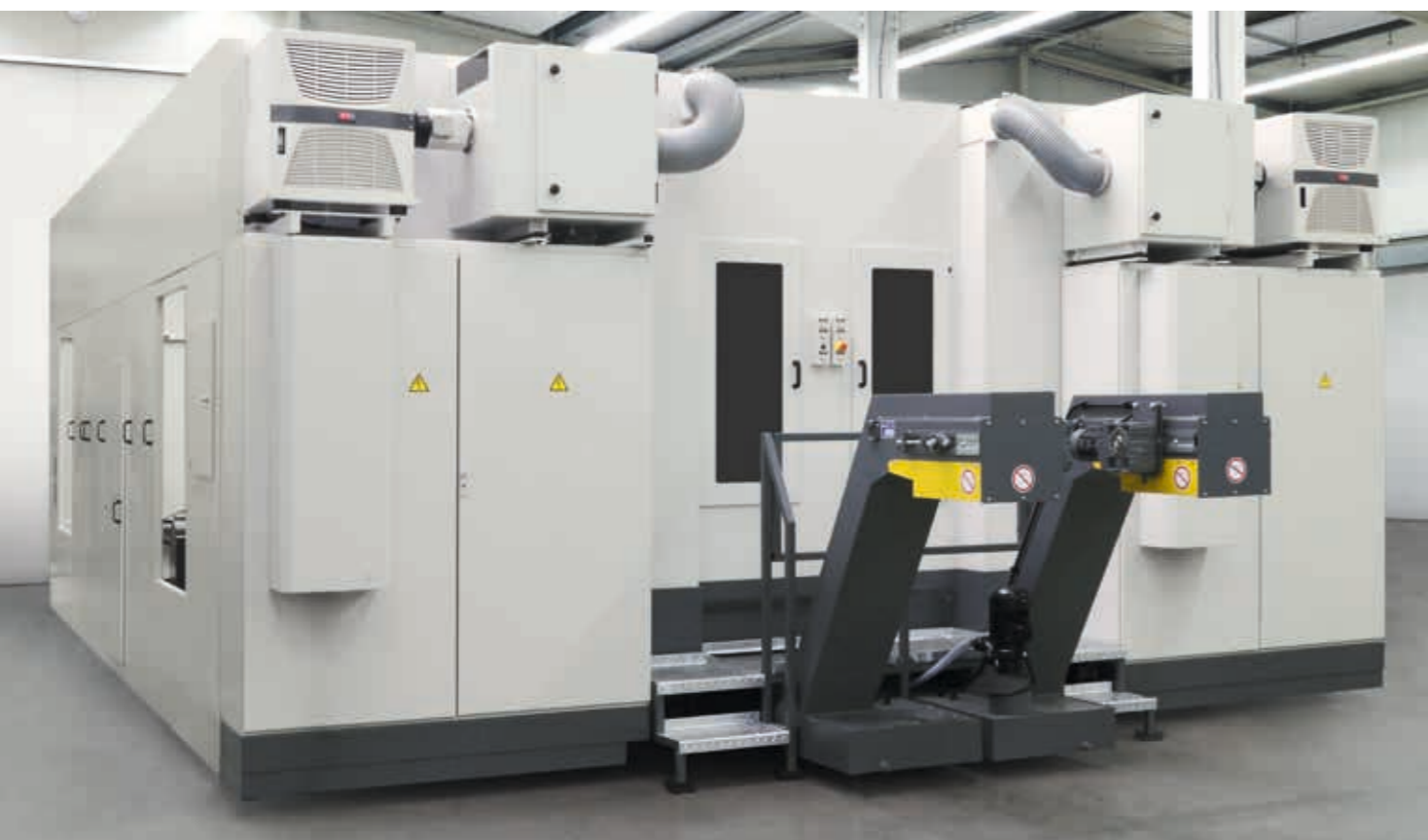
For machining long profiles, two travelling columns are set up opposite one another, each with its own control cabinet and its own controls
