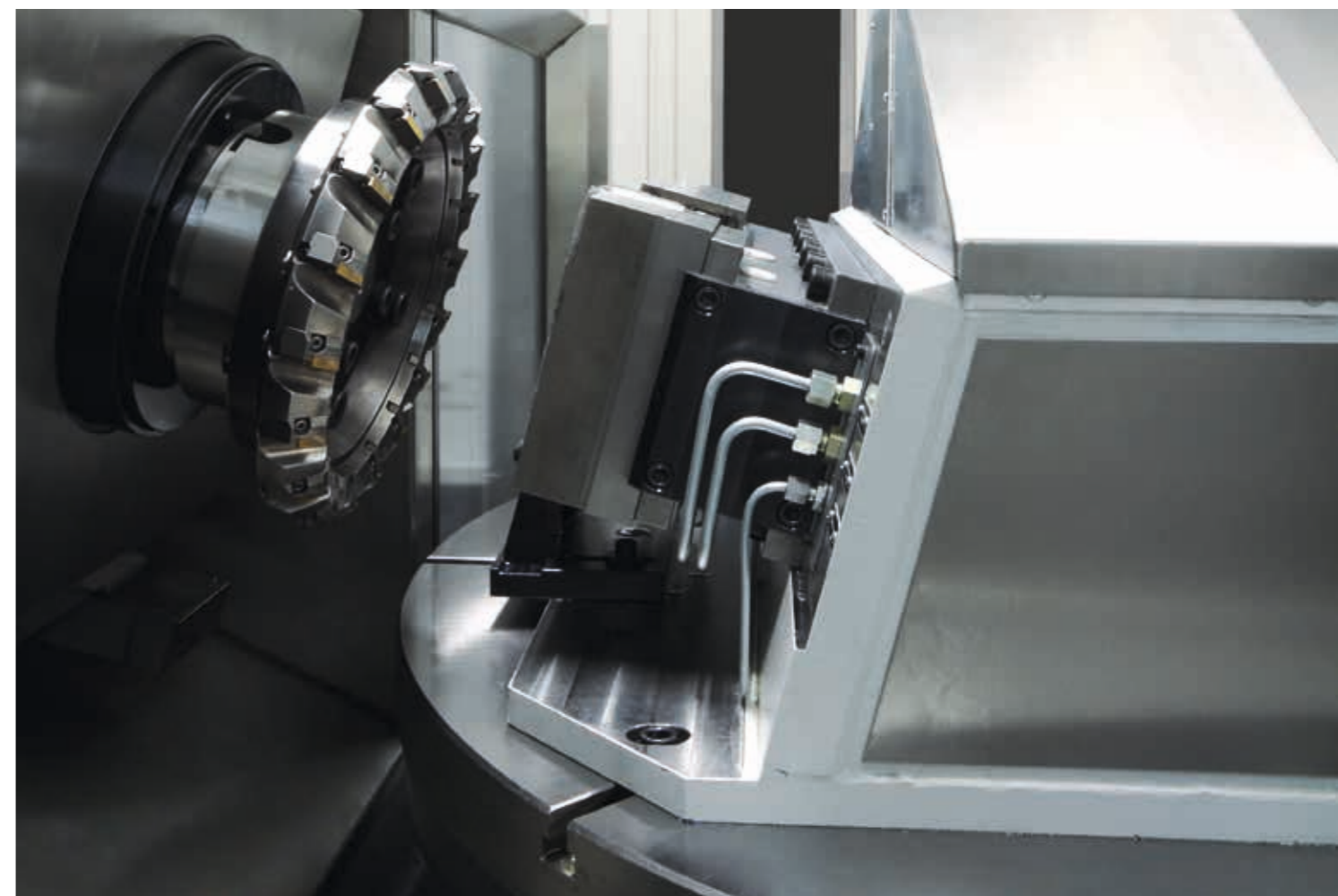
The slightly inclined machining position allows a good chip flow to be achieved during milling and ergonomic handling of the workpiece assembly
