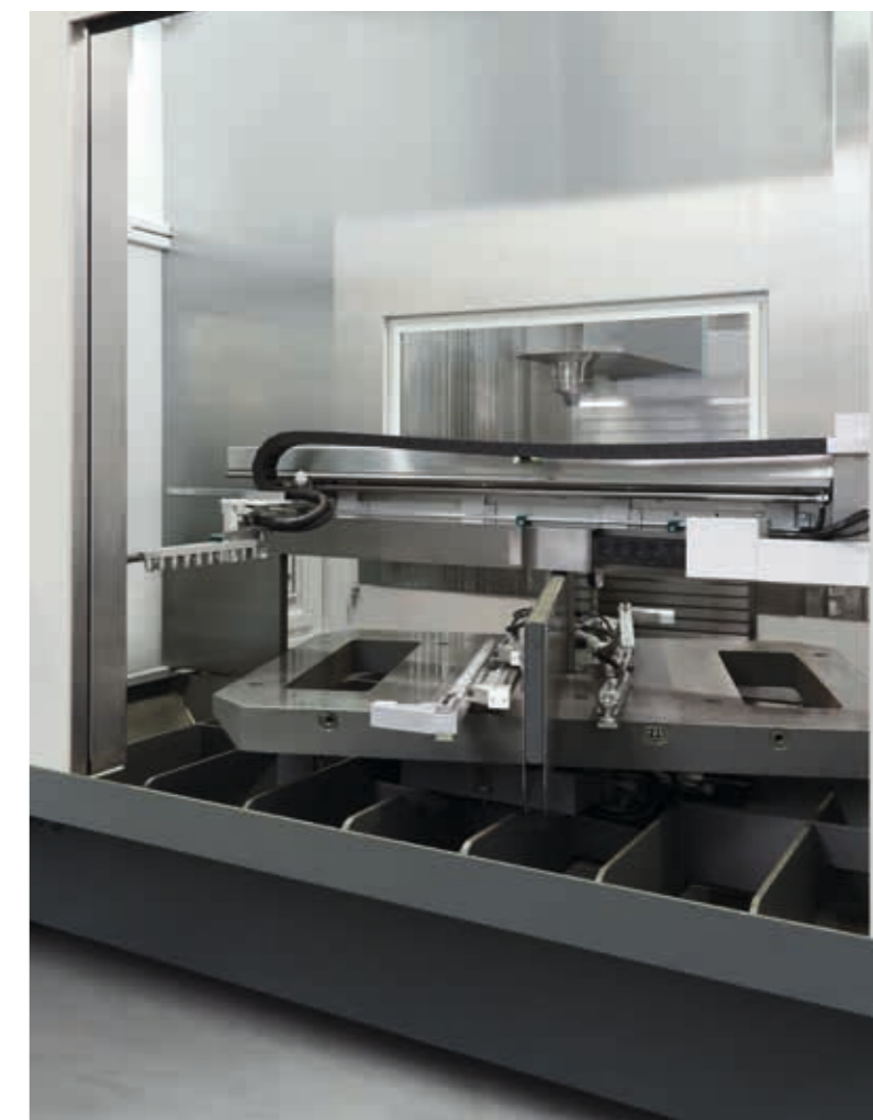
By pivoting the indexing table through 180° the ready-machined workpiece is rotated into the setup position while the next raw workpiece is simultaneously rotated into the machining position
