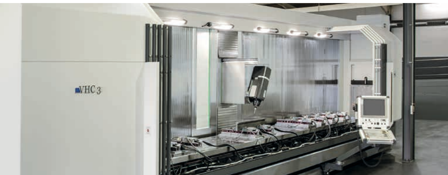
The machining centre with tilting spindle head is used for milling long steel girders and additionally for welding bolts
