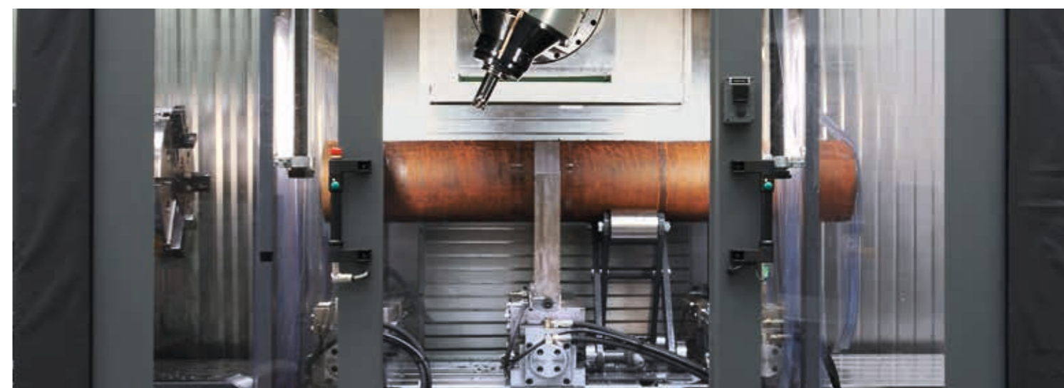
Using the movable rotary table, the pipe ends can be held and the pipes can be rotated into position for the introduction of radial drill holes
