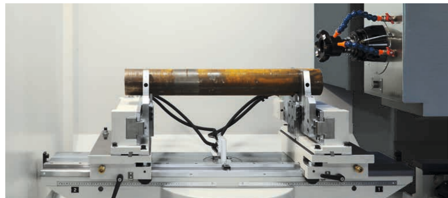
The distance from the centring clamp, which can be moved and clamped manually, is adapted to the length of the workpiece
